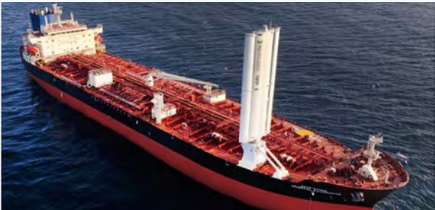
Wind-assisted propulsion system "Wing Sail"
